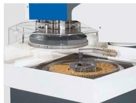
AC 535-F process area with swiveled out upper working wheel
