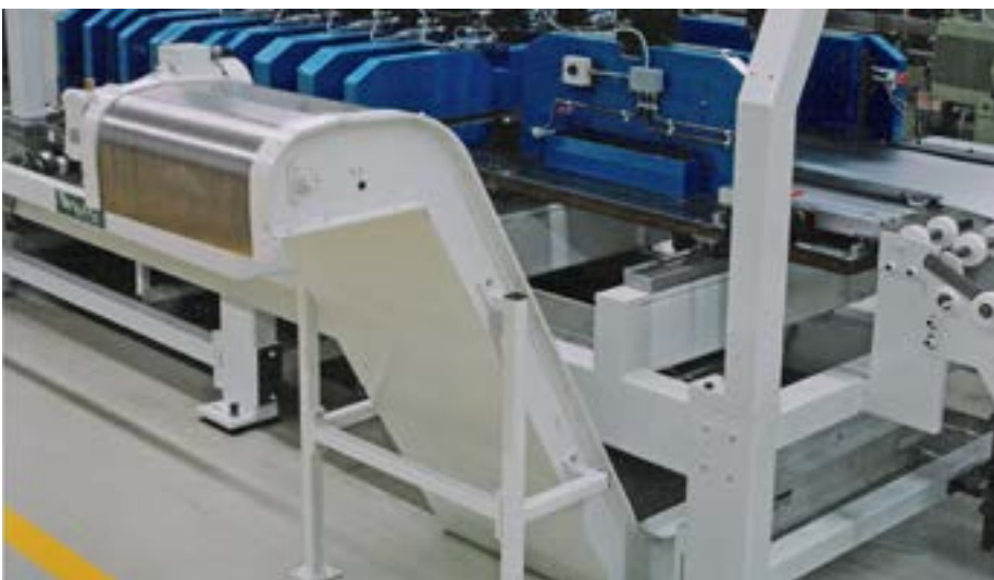
Slide conveyor mounted under a stamping machine to carry off the scrap metal.
