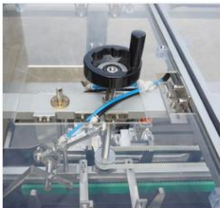
4 Hand wheel for easy change over different size carton
