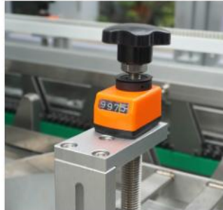
5 Visual dial gauge for easy change over different size carton
