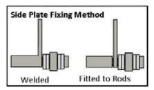
All available specifications can be supplied with side plates and cross flights in various combinations of height and design enabling elevation or product separation as required by the application.
