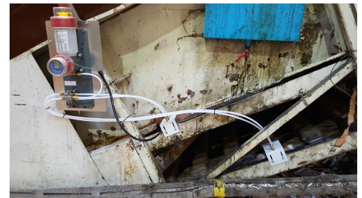
4 brushes applying oil to paper recycling conveyors
