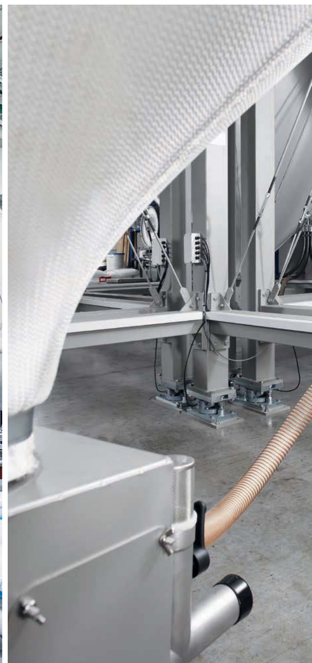
Flexible silo plant for fresh foamed EPS – Volume per storage silo approx. 90 m 3
