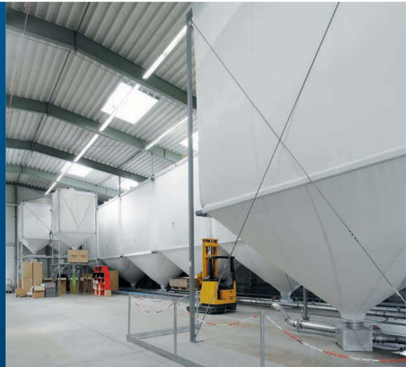
Flexible silo plant for fresh foamed EPS – Volume per storage silo approx. 90 m 3
