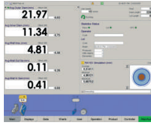
Main screen showing, among others, line schematic, status and instrument view, as well as characteristics view.
