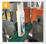
To safeguard product quality, the machine can be equipped with print and label presence checks combined with a label return for misprinted labels and a product reject station.
