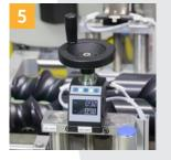
Electronic position indicators and motorized height adjustment support quick format changes and enable very short set-up times.
