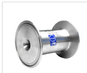
Example nozzle with PTB calibration
