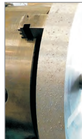
contact wheel core after the final turn off - ready for new coating
