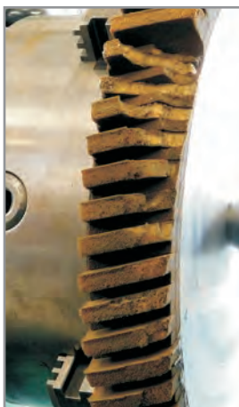
Contact wheel with an old coating made of lamellae of foamed Vulkollan®
