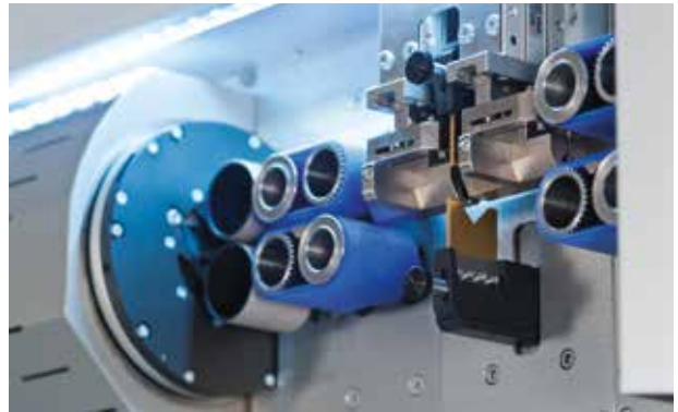
▲ Kappa 331 Universal/coax machine with split guide
