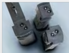
Inserting balls to seal holes
