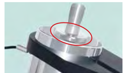
Load cell contact area, via which force is transmitted
