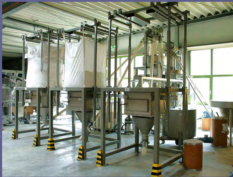
Multiple big bag emptying stations for different products (multicomponent dosing station)
