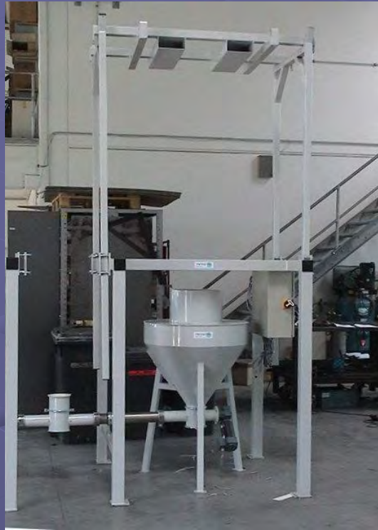
Emptying station with separate hopper and spiral conveyor.
