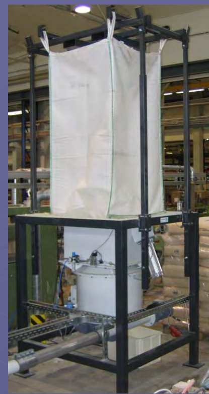
Emptying station with combined discharge and metering device
