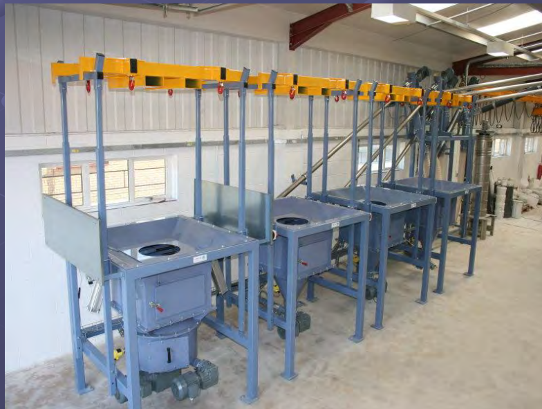
Multiple big bag emptying stations for different products (multicomponent dosing station)
