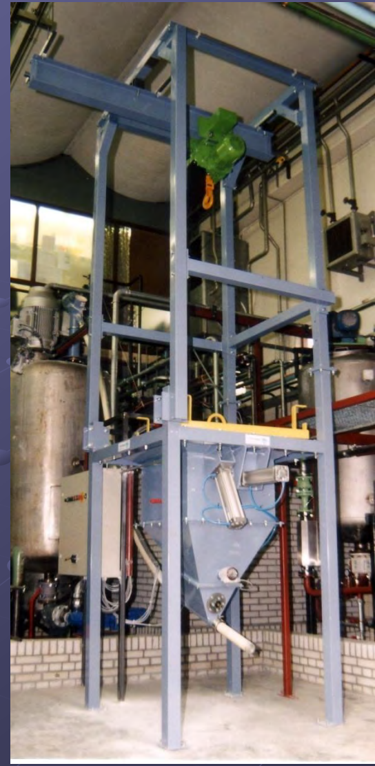
← ↑ Loading of the station using a crane runway which is integrated within the emptying station
