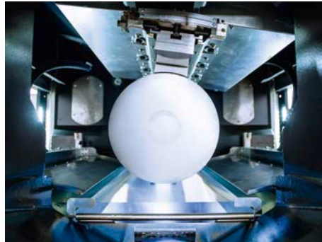
Optimized work piece rocking for higher wafer quality
