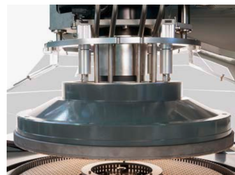
Leveling device enables loading and unloading in the gap
