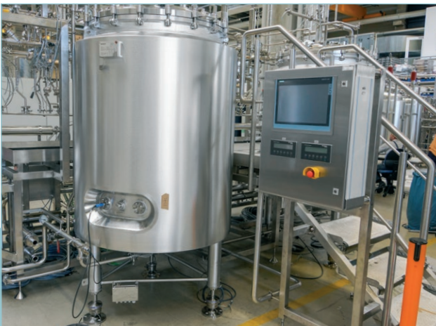
The installation of the weighing module was particularly simple thanks to the integrated height adjustment of the Novego.
