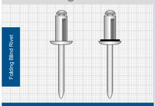
The wide spreading of the closing head of folding blind rivets ensures a uniform distribution of the forces involved similar to that of the ARCO® body-bound blind rivet to be seen on ▶ page 76 so that soft or brittle parts, in particular, are burdened less and the surfaces are protected. They can also be used on parts that are not flat, as the tabs of the closing head adapt to the contours.
