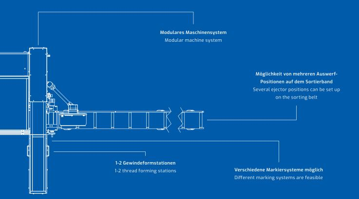
The new FlexPunch series features a very flexible and modular system. Each machine can be adapted to the customer's individual requirements via individual components. The FlexPunch compact is the smaller version of the two and is particularly suited for production sites with limited space.
