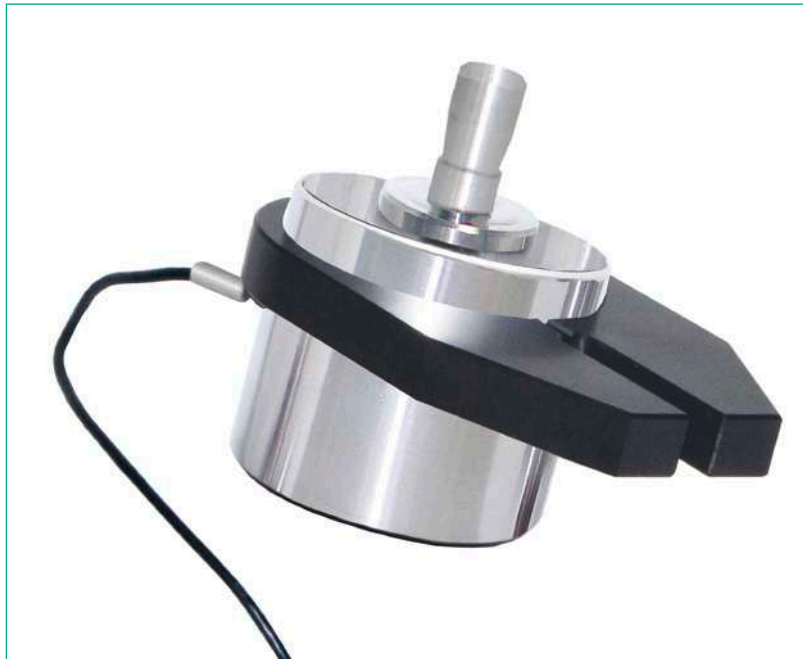
Figure 1.1: Fitting the carrier on the load cell
