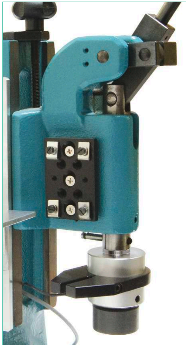
Figure 1.4: Displacement measuring system on the press
