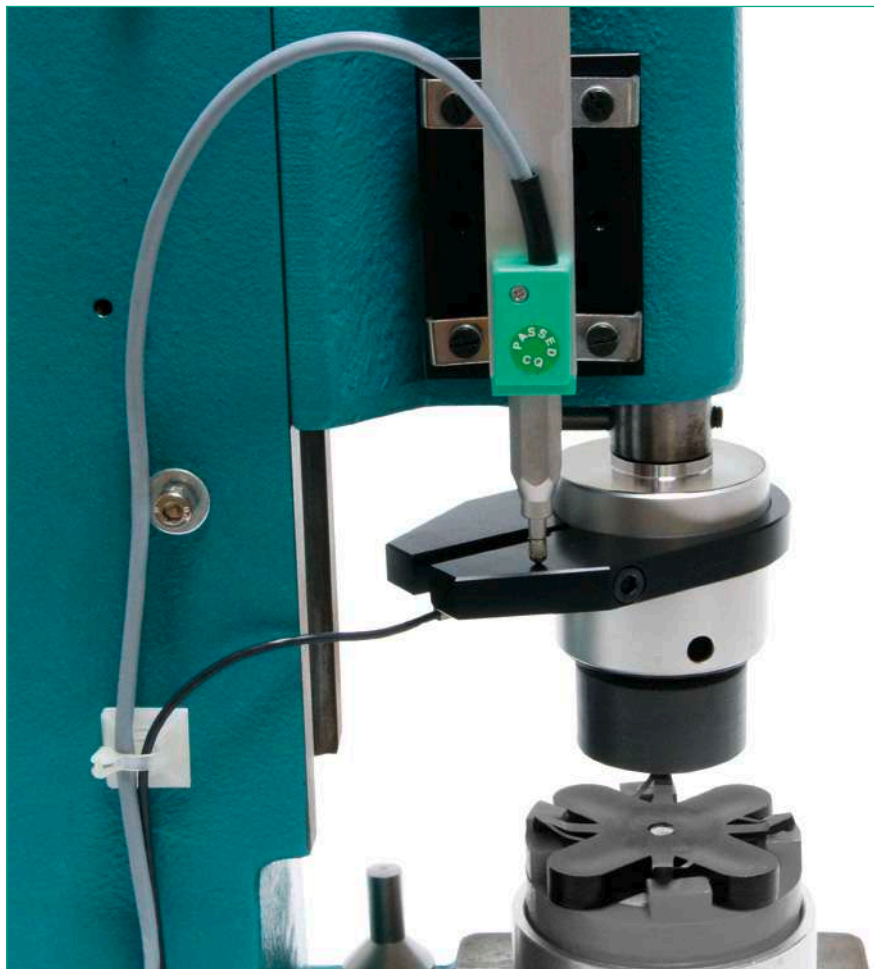
Figure 1.5: Displacement measuring system in the raised position
