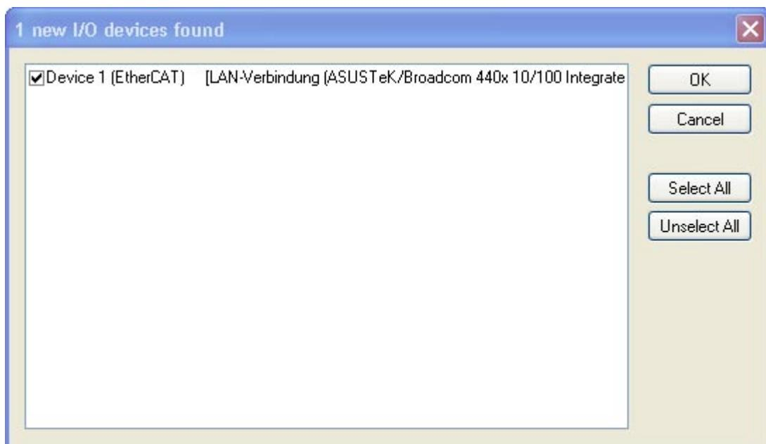
After confirming the following dialogue with “Yes”, all connected devices should be located. In this case, the EtherCAT master (device 1), a Beckhoff bus terminal with I/O modules and the TWK displacement transducer (Magnosens).
