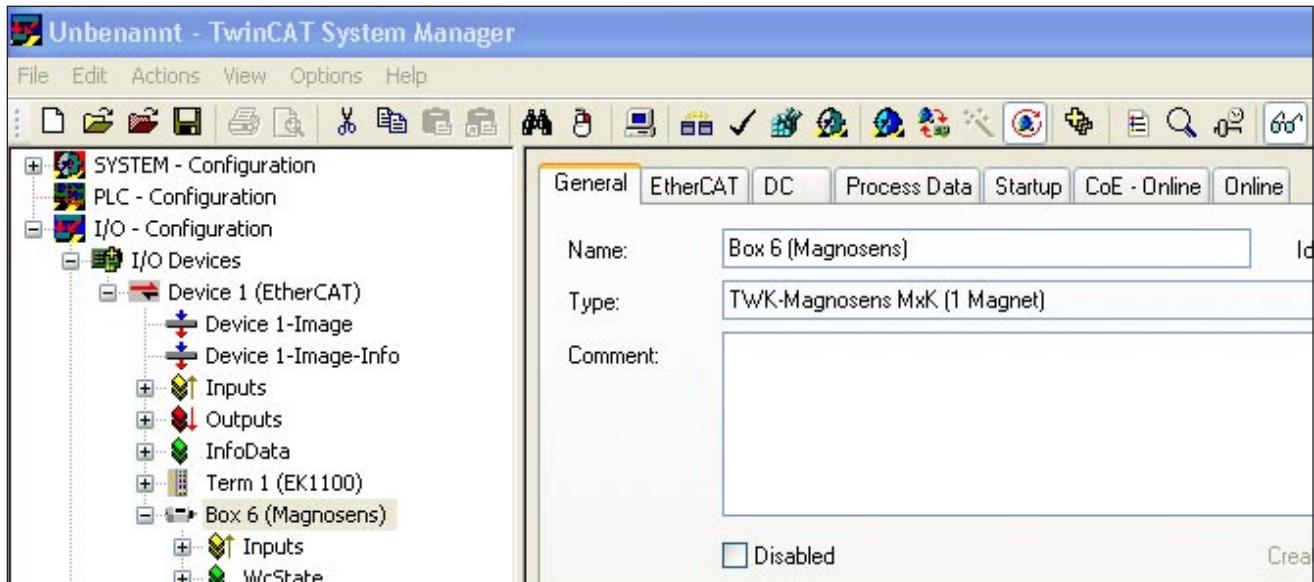
The CoE online register accesses the parameter and diagnostic data. All parameters identified with "RW" can be changed. The description of the parameters can be found in Chapter 4. Do not forget to subsequently save the parameters in a failsafe manner via parameter 200C<sub>h</sub>.
