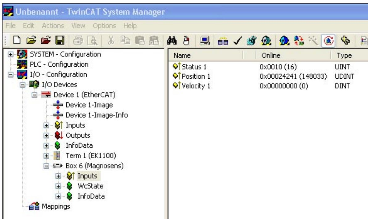
If you click onto the Magnosens itself instead, the following screen's register takes you to the displacement transducer's configuration and parameterisation.
