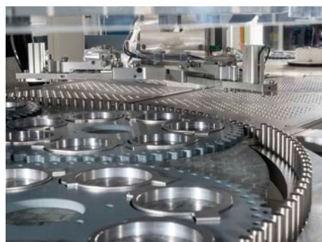
View from the process area into the Twin Loader – for shortest carrier exchange time
