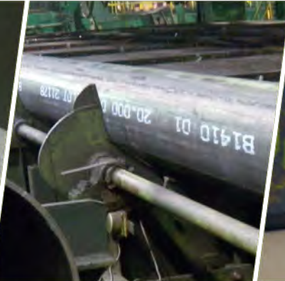
Steel pipe marked with SCP-800 white pigmented ink.
