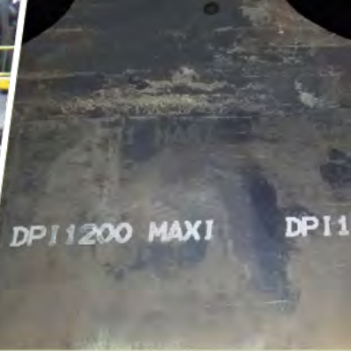
Steel plate marked with SCP-899A after 30 hours at 1000 degrees F.
