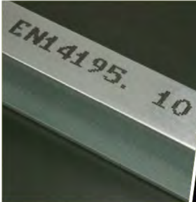
Aluminum 2x4 marked with SCP-700 after processing.
