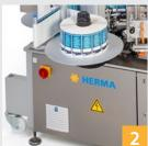
Handwheels with digital position indicators enable users to replicate optimal settings at any time.
