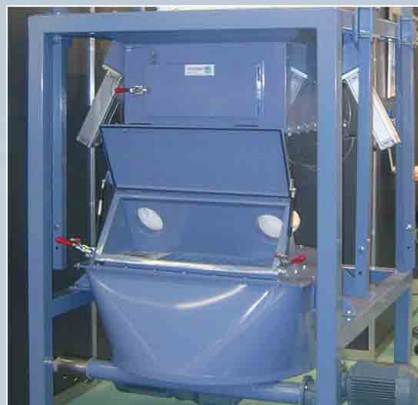
Big-Bag Emptying station with additional chute for emptying sacks
