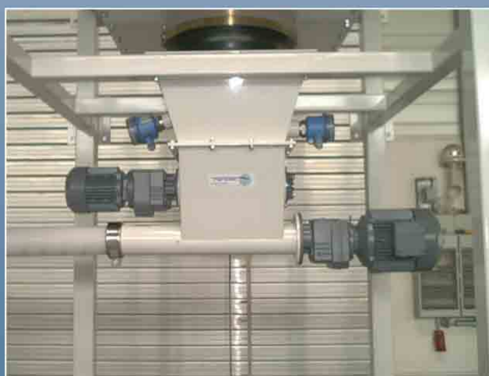
Material collecting hopper type FW with agitator
