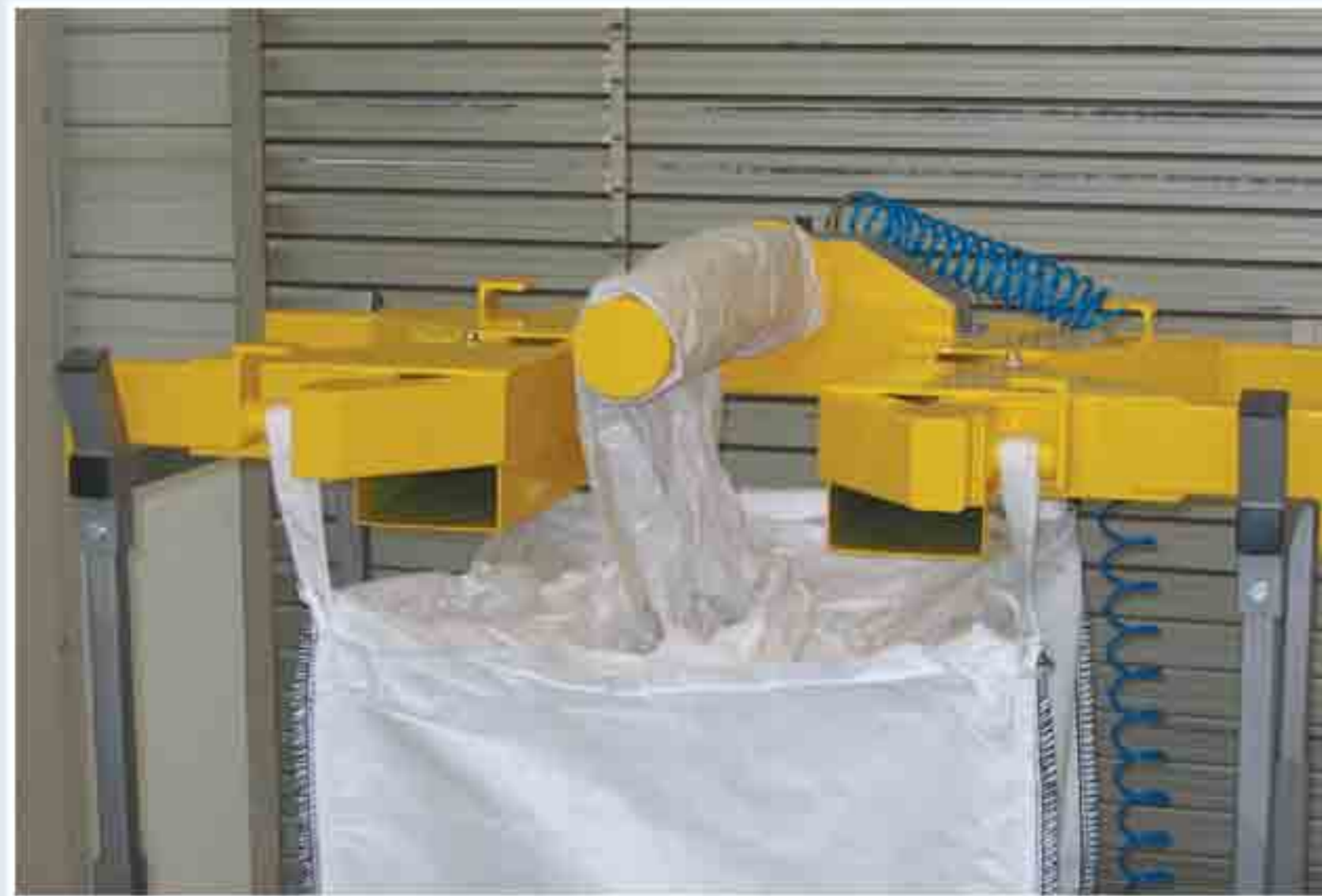
Big-Bag cruciform with device for automatic spooling of the Big-Bag inliner
