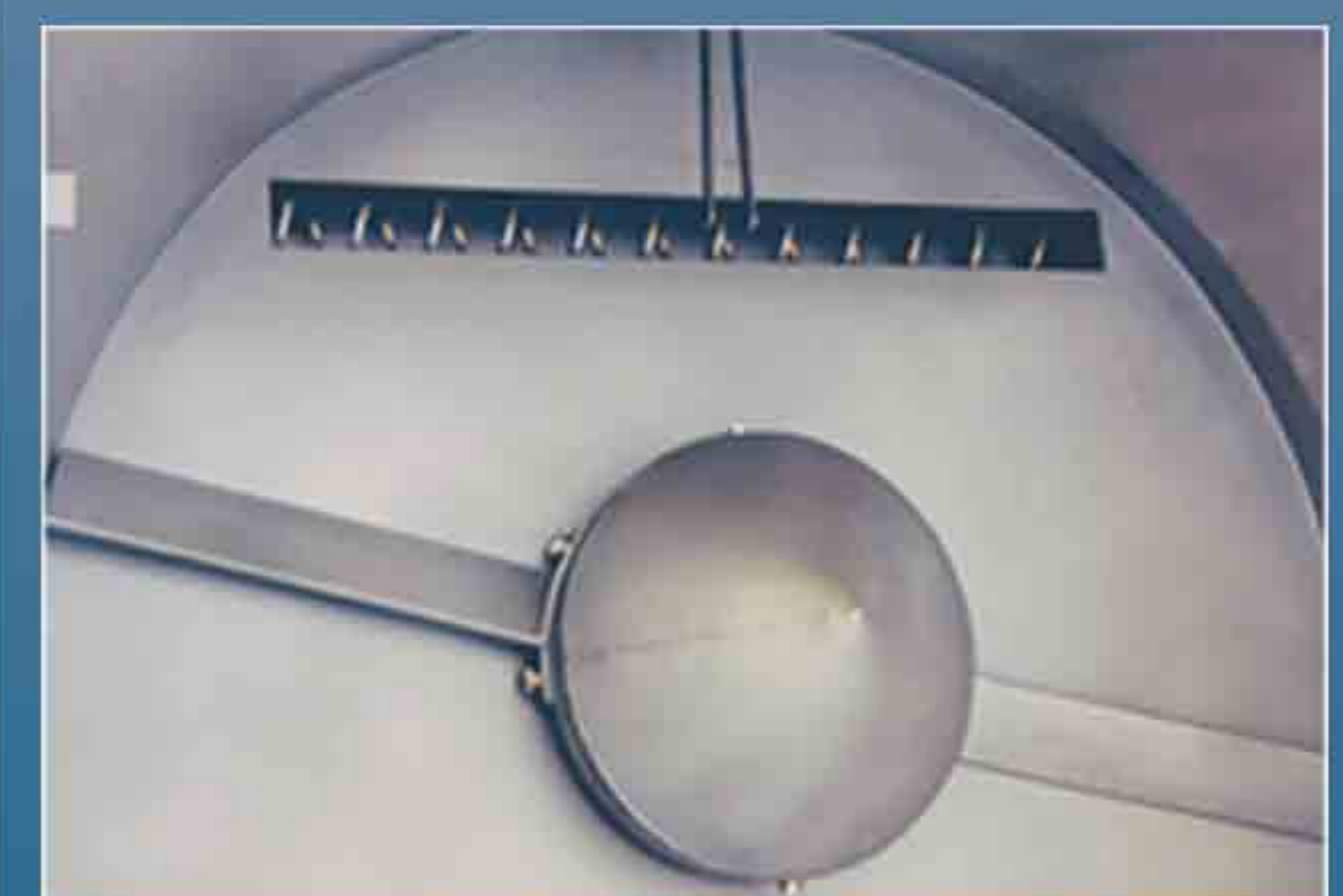
Collecting hopper type DZR for bad flowing and bridge building bulk materials – cylindrical hopper with flat bottom and rigid rotating blades.
