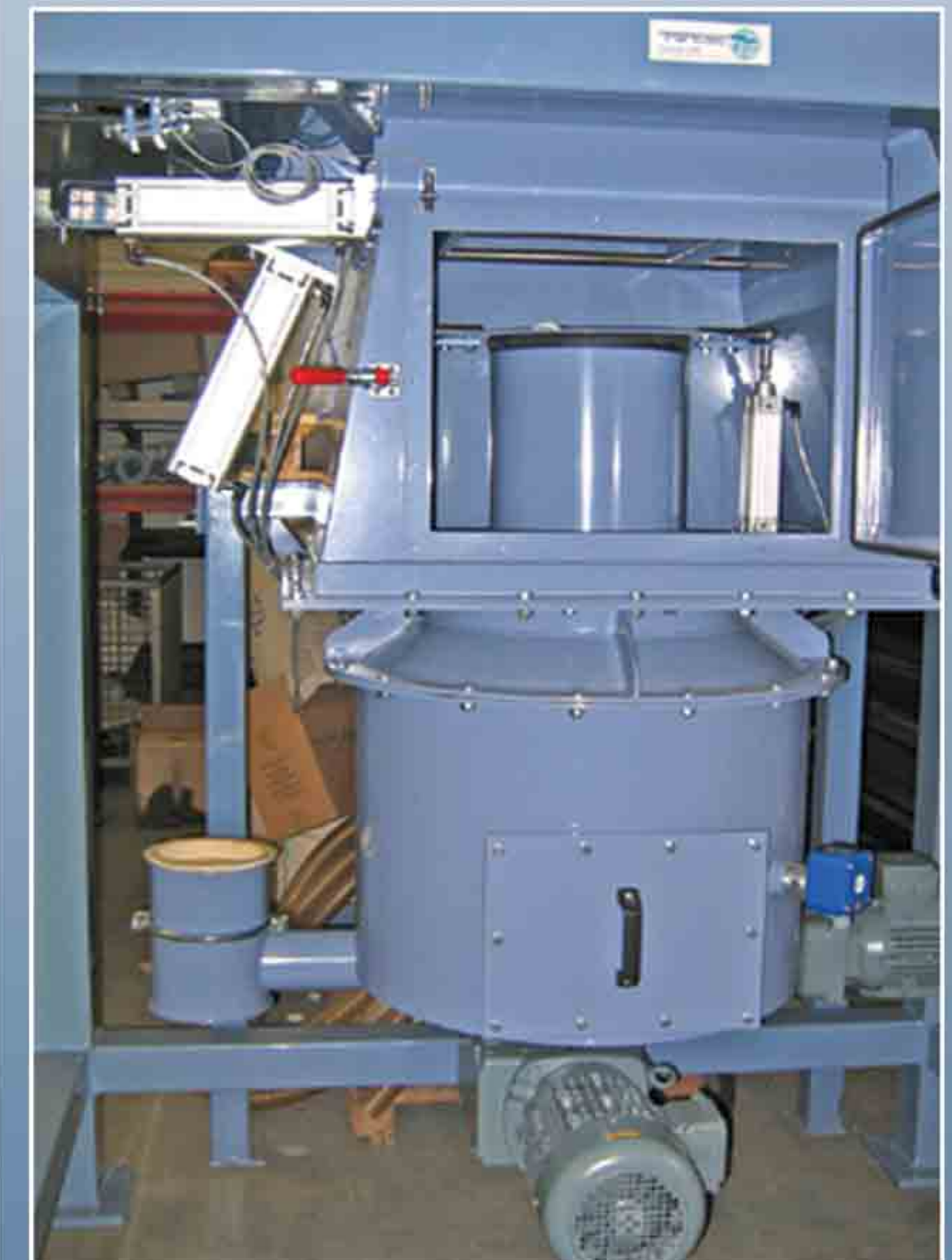
Collecting hopper type DZR for bad flowing and bridge building bulk materials – cylindrical hopper with flat bottom and rigid rotating blades.
