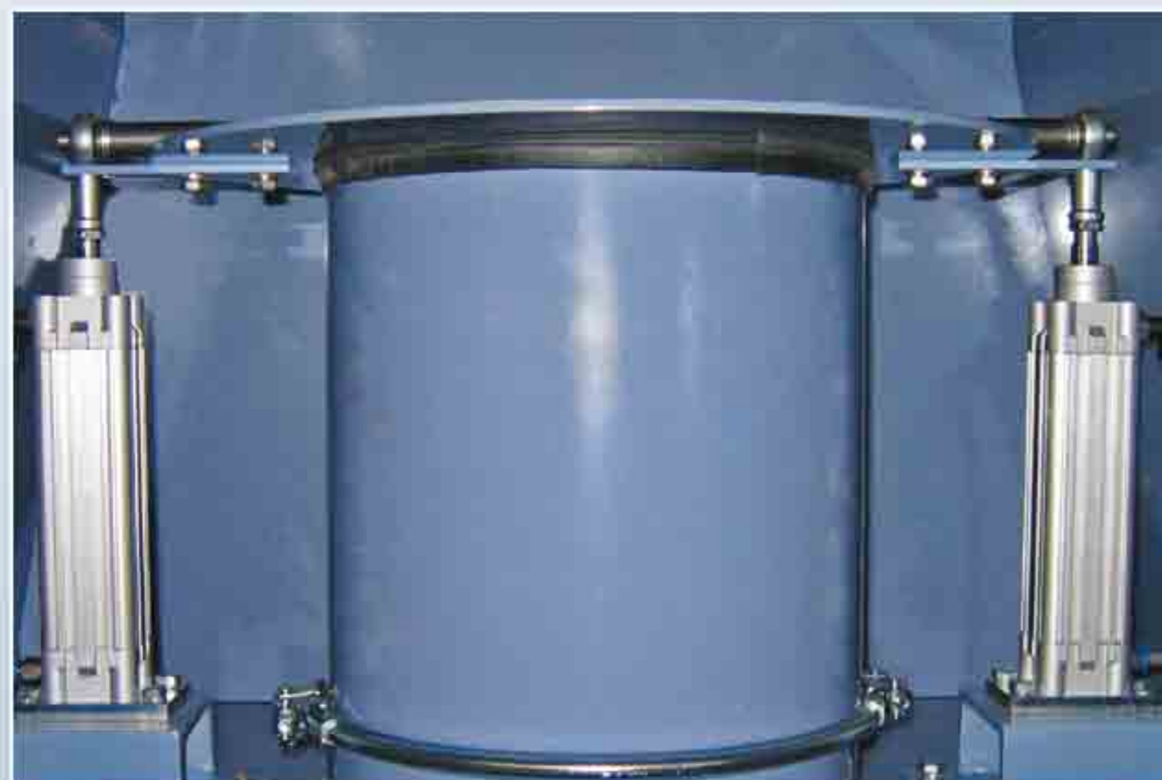
Device to clamp the outlet spout of the Big-Bag
