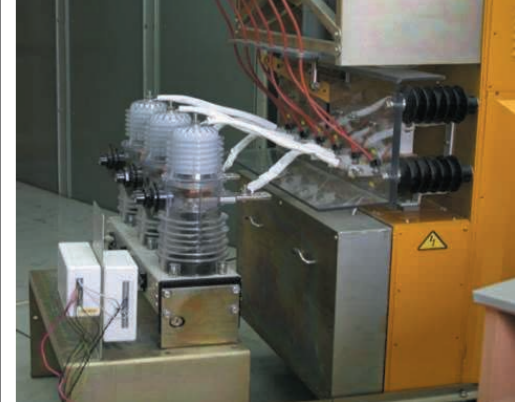
▲ Unit for life testing with rated current of up to 1,600 A
