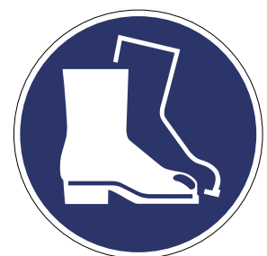
Use foot protection (ASR A1.3)
