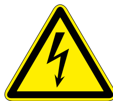
Warning against electrical voltage (ASR A1.3) Motif number | SW12
