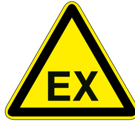
Warning of explosive atmosphere (ASR A1.3)
