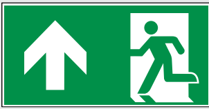
Escape route straight ahead, through the door, go up (ASR A1.3)
